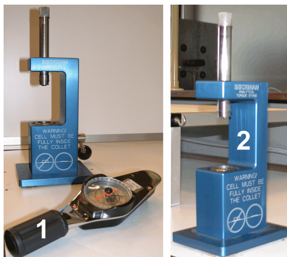
Figure 6.10: Torque wrench (1) to tighten the assembled cell and a collet (2) to hold the cell in place.
